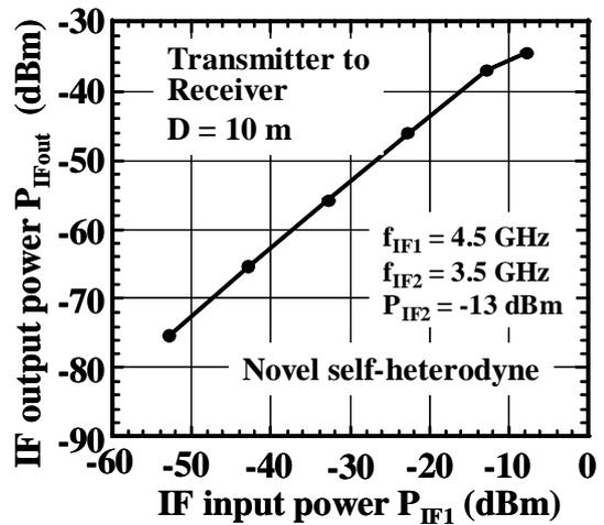
Fig.8 IF output power  $P_{IFout}$  in Rx vs. IF input power  $P_{IF1}$  in Tx.
