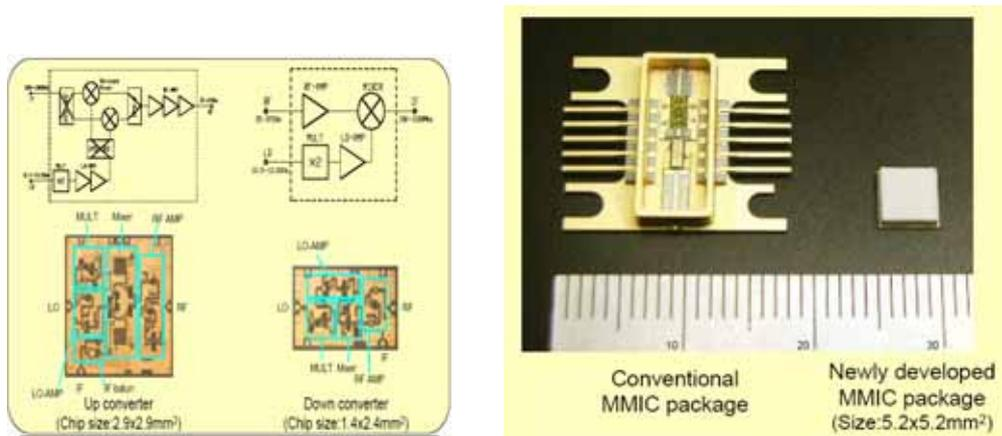
Fig. 5 Block diagram of the up and down converter and down-sized MMIC package.
