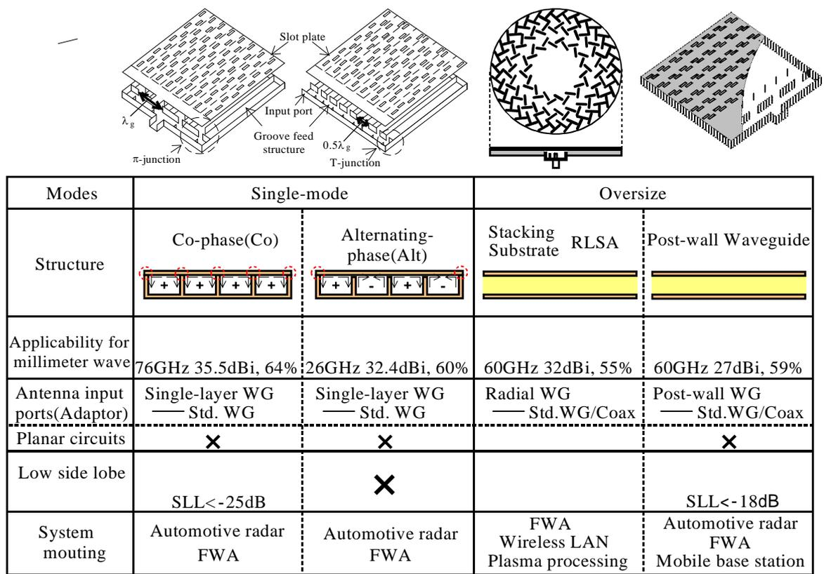
Fig. 1 Four types of single-layer slotted waveguide arrays, interfaces and applications
