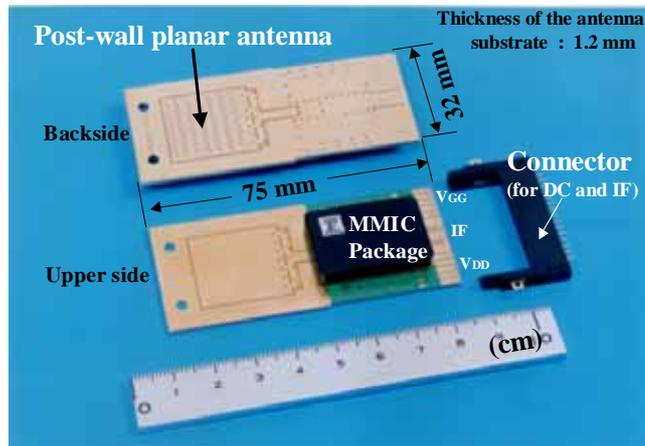
Fig.6 Completed cost-effective 60-GHz module with a post-wall planar antenna. MMIC package  $30 \times 21 \times 6 \text{ mm}^3$ . The total size of the module  $75 \times 32 \times 1.2 \text{ mm}^3$ .
