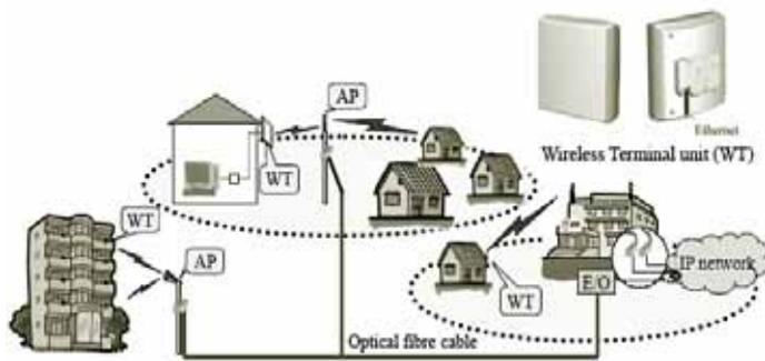
**Fig. 3** Configuration of Wireless IP Access System (WIPAS)
