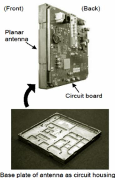
**Fig. 4** Assembly of Wireless Terminal (WT) and an alternating-phase fed single-layer slotted waveguide array..
