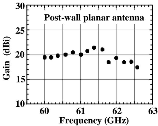
Fig.7 Measured frequency characteristics of the antenna gain.
